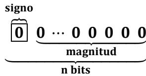
$$SM(Z, n) = \begin{cases} Z_{SM,n} = BIN(|Z|, n-1) & \text{con signo} = 0 \text{ si } Z \geq 0 \\ & \text{con signo} = 1 \text{ si } Z < 0 \end{cases}$$
